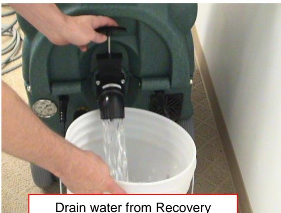
Drain water from Recovery Tank
