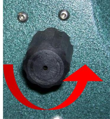
To increase the solution pressure, turn the regulator knob clockwise.
