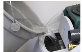
Pour 2 or 3 gallons of clean water into Solution Tank
